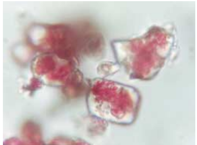
Fig. 1: As seen by microscope, the brilliant red cadmium in an inclusion pigment is completely enclosed in stable zircon crystals.
