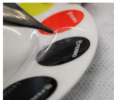
Fig. 3: Removal of the strippable coating 80 2039
