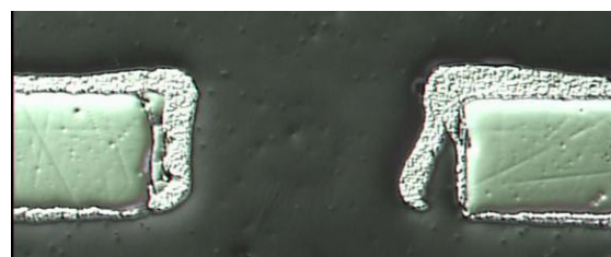
Figure 1: Cracks in the PUM through-hole metallization cause huge fill factor losses.
