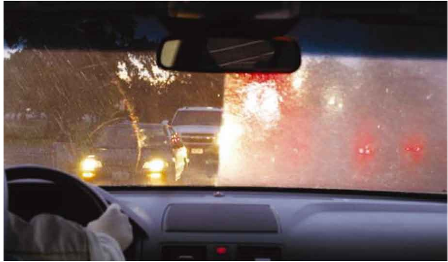
Figure 13. Treated and Un-treated Automotive Glass in a Rainstorm 6
