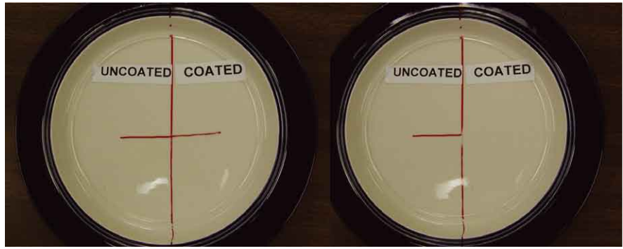
Figure 12. Permanent Marker Pen is Removed by Scotch Tape on Coated Glass 6
