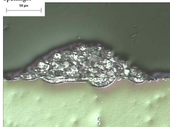
Fig. 3.7 Optical microscope cross-section of fine line printed paste.
